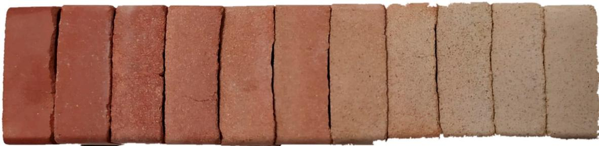
**Figure 3.** The color of the different families of samples composed of clay and biomass bottom ashes. 100% clay (0A10C) on the left; 100% biomass bottom ash (10A0C) right.
