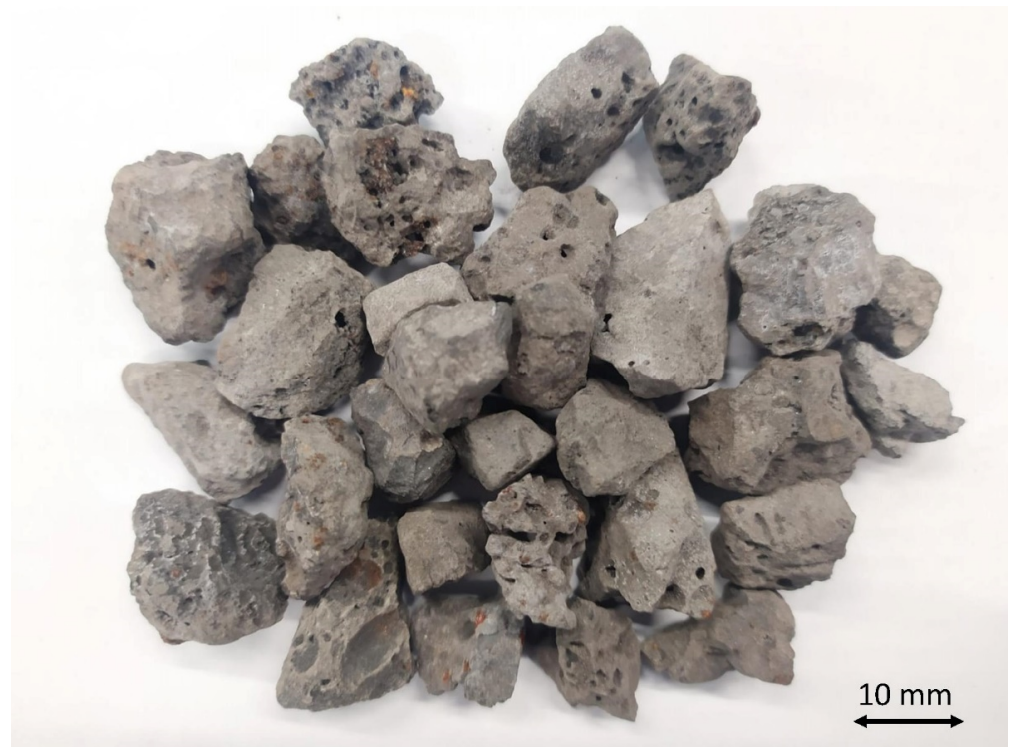
Figure 3. Image of electric arc furnace slags.
