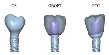
**Figure 4.** Three different implant-supported crown designs: GS, screw-retained crown; GBOPT, cemented without finishing line; GCC, conventional cementation with finishing line.
